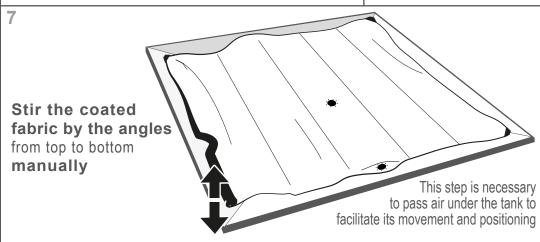
Shake and spread correctly the tank to remove all the folds
