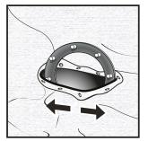
STRETCH WITH CARE without tools, in order to pass inside the counterflange with its seal
