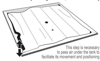
8 Shake and spread correctly the tank to remove all the folds
