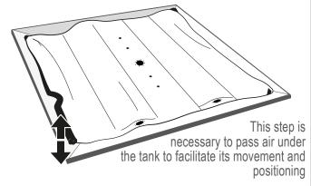
9 Shake and spread correctly the tank to remove all the folds
