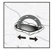
STRETCH WITH CARE without tools, in order to pass insite the counterflange with its seal
